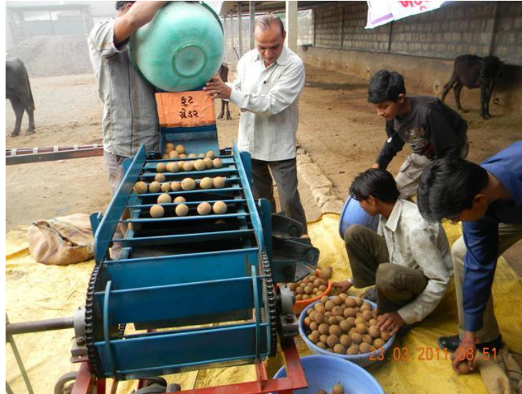
Plate 3.3 : Flapper type grader
