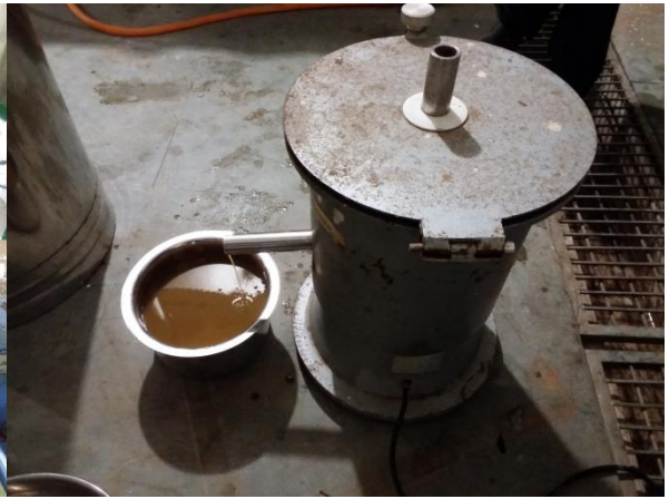
Separation of pectin extract using basket centrifuge
