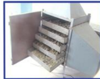
LOADING OF DRYING TRAYS IN THE DRYING CHAMBER.
