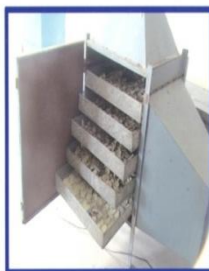
LOADING OF DRYING TRAYS IN THE DRYING CHAMBER.
