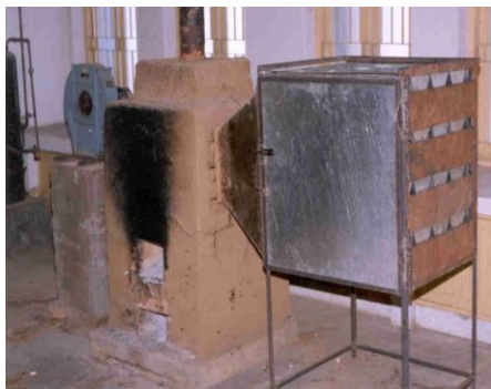
Waste fired dryer
