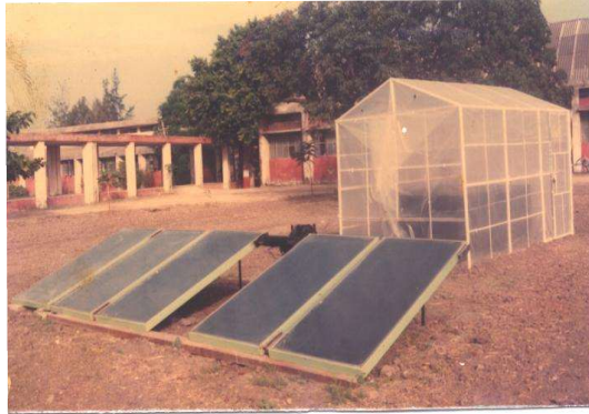
Solar Dryer cum Green House
