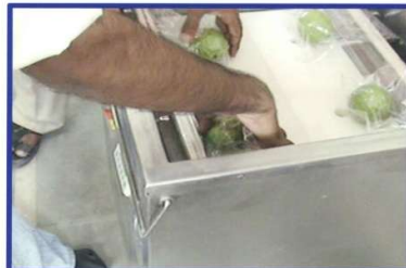
PACKAGING OF GUAVA FRUITS USING VACUUM PACKAGING MACHINE
