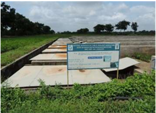
Soil Conservation Field Laboratory (Runoff- Soil Erosion Measurement Structure)
