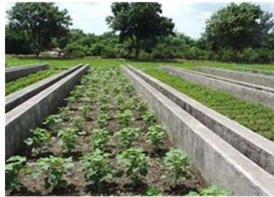
Soil Conservation Field Laboratory (Runoff- Soil Erosion Measurement Structure)
